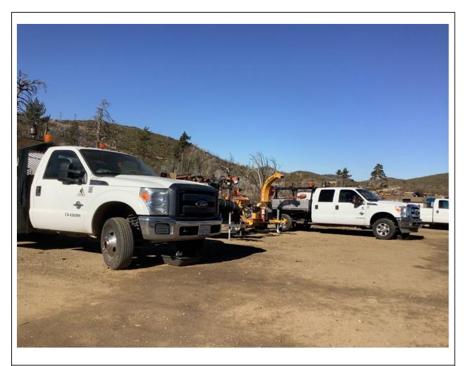
**Photo 5:** Drip pans were observed under staged vehicles and equipment at Shrine Camp Staging Yard (C 440) to prevent leaks or spills from being discharged onto the ground in accordance with the SRNP and MM PHS-2.
